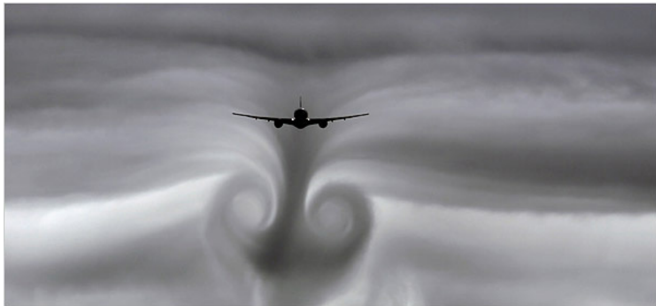
Wake Turbulence induced by a plane after takeoff
