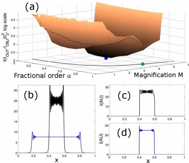
Fig. 3. (Color online) Reconstruction error of a rectangular signal. (a) Error as a function of fractional order  $\alpha$  and magnification  $M$ , (b) field at recording device for optimal configuration for free-space propagation (black, narrow profile) and single-lens configuration (blue), (c), (d) reconstructed (readout) output fields for (c) free-space and (d) single-lens configurations.
