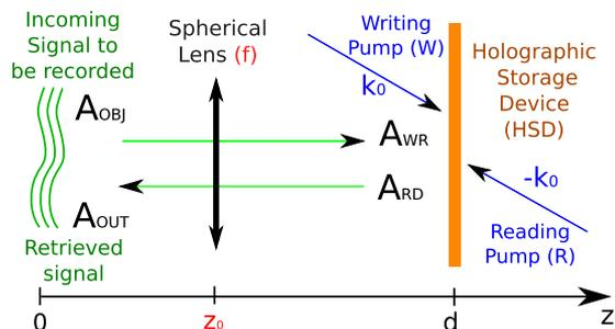
Fig. 1. (Color online) Reflection-type setup for quantification of holographic storage efficiency. In the optimal configuration, a thin spherical lens (position  $z_0$ , focal length  $f$ ) minimizes the reconstruction error.
