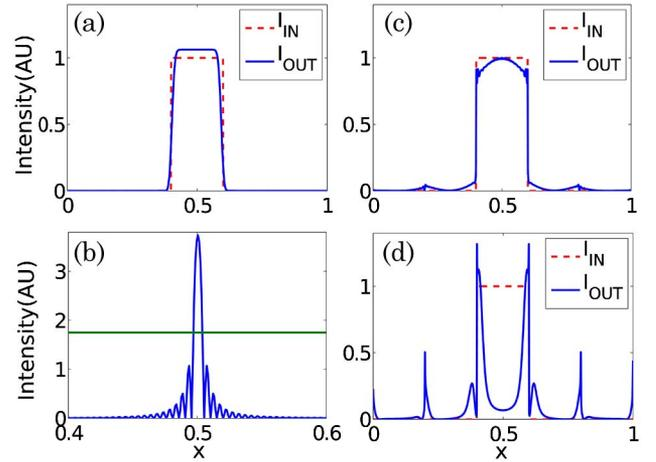
Fig. 2. (Color online) Input (dashed red) and readout (blue) simulation results for a rectangle signal. (a) Reconstruction of real-space hologram ( $\alpha = 0$ ). Diffusion effects on the storage device induce reconstruction error on the edges. (b) Fourier transform of the rectangular signal. Green line shows the saturation level of the device. (c), (d) Reconstruction of Fourier-space hologram ( $\alpha = 1$ ) after (c) diffusion and (d) saturation on the device.
